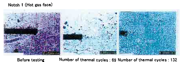
Fig.16 Optical microphotographs of crack growth from Notch 1 of shroud segment after 69 and 132 thermal cycles.
