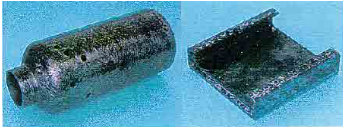
Combustor liner Shroud segment
