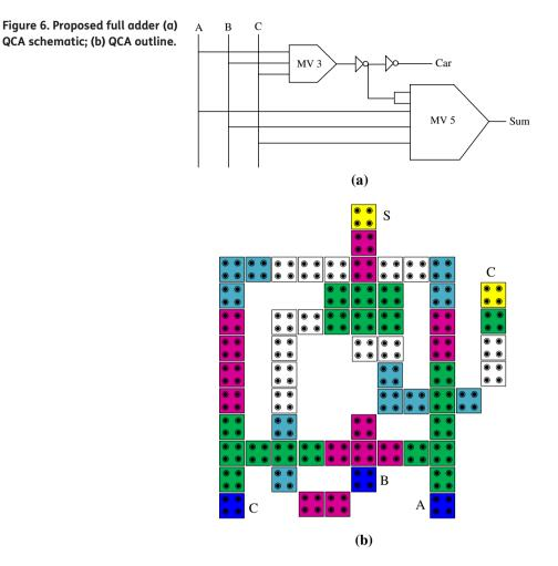
The designed binary full adder is carry out in single layer and only 63 cells with four clock levels is used to produce accurate outputs shown in Figure 6. In contrast to previous model the designed adder developed in considerable progresses in terms of area and cell complexity, wire crossing, and has an identical organization in terms of clock delay. Simulation outcomes part compares all earlier outlines and displays the achievement of the proposed layouts.
