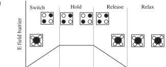
Figure 3. Four phase clocking mechanism in QCA.
