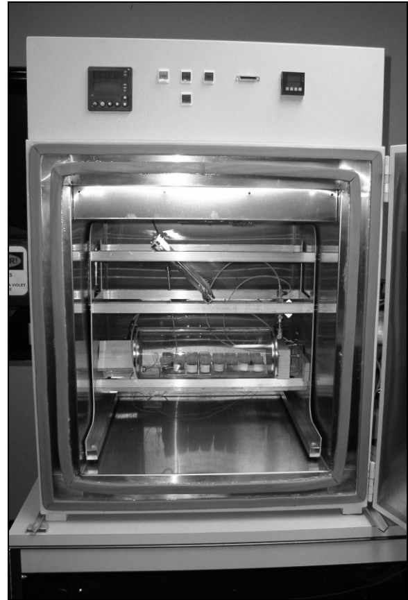
Figure 1. The SHOT Mars simulator. Samples are contained within the 6 liter quartz cylinder. Simulated sunlight is reflected onto the samples via a movable, front-surface mirror. The xenon-arc light source is connected at the left side of the simulator (not shown).
