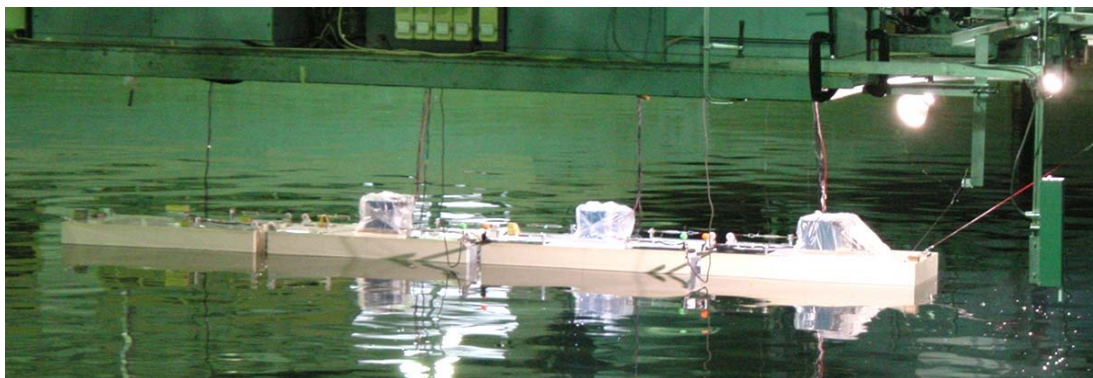
Fig. 8 Model basin test using four floating body units of 1/30 scale models
