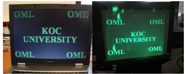
Fig. 4 The original image with green letters on the black computer screen (left) and the laser scanned image on the A4 size white screen (right)
