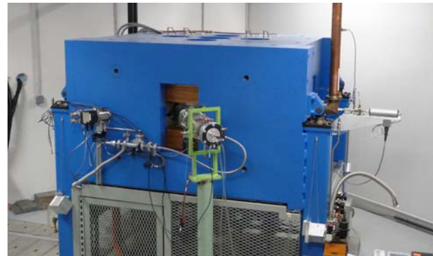
Figure 1: Picture of the TR24 cyclotron installed at IPHC in Strasbourg. The water cooled beam dump provided by ACSI is visible at the end of the beam pipe.
