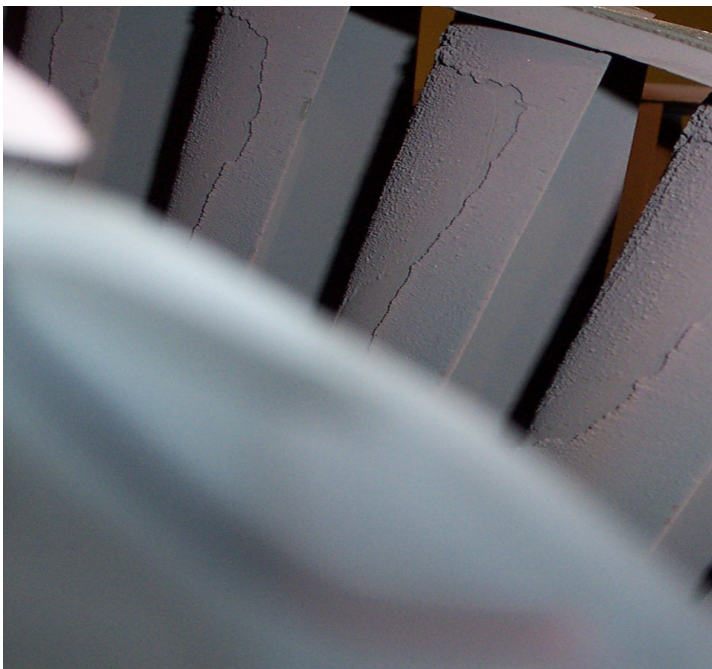
Figure 2: Generating station deposit accumulation on turbine blades, courtesy of ALSTOM
