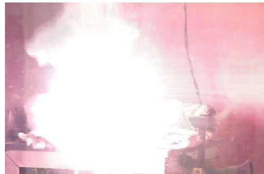
c). Large flame burst from wire insulation 433 ms later.
