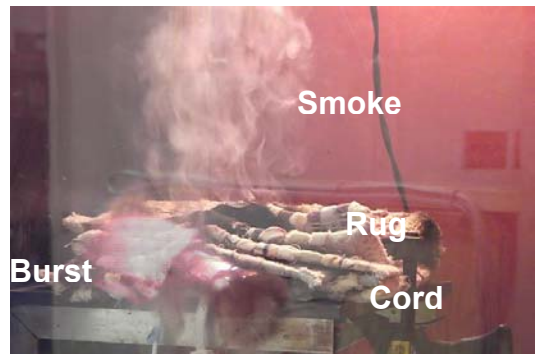
a). Initial flame burst from gases produced from PVC wire insulation after 100 h.
