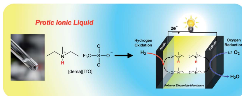
Fig. 4 Application of ILs as proton carrier in a non-humidifying intermediate temperature fuel cell. Reproduced from ref. 71 with permission from The Royal Society of Chemistry.
