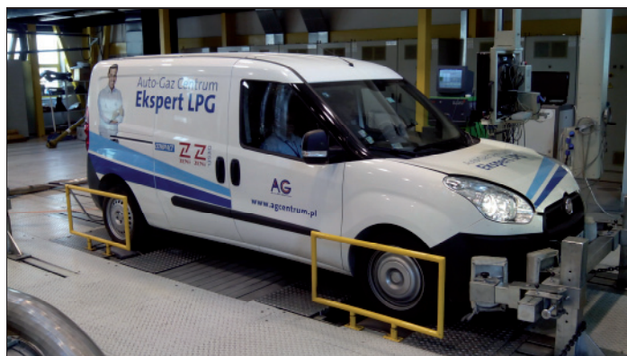
1: Fiat Doblò on the chassis dynamometer
