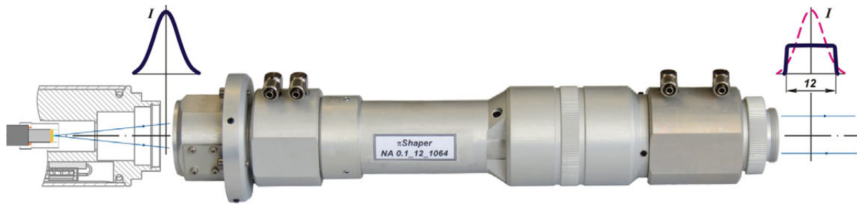
Figure 3 Conversion of divergent Gaussian beam from fiber to collimated flattop.
