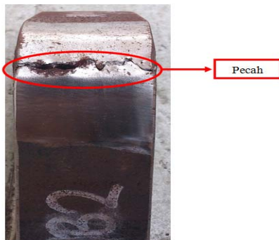
Figure-13. Surface condition of specimen of wet-welded joint using E-7018 electrode after face bend test.
