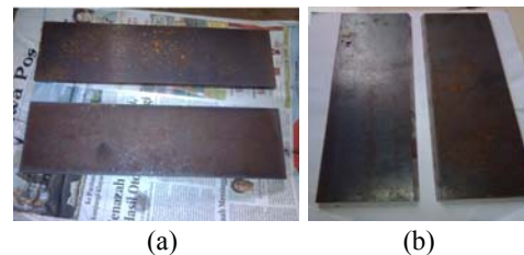
Figure-1. Sample preparation (a) Cutting out of the sample of ASTM A36 steel, (b) beveling.
