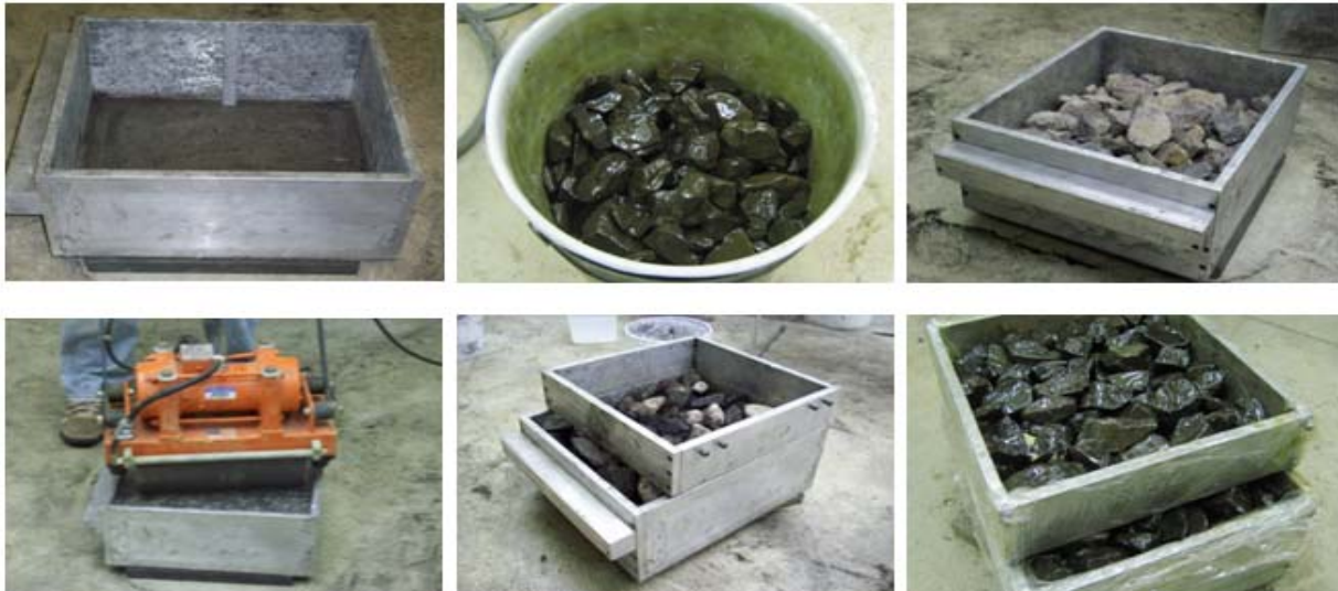
Figure 3 - Stages of ballast preparation, compaction, and loading upper ring.
