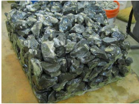
Figure 8 - Single block removed from direct shear test apparatus after shearing.
