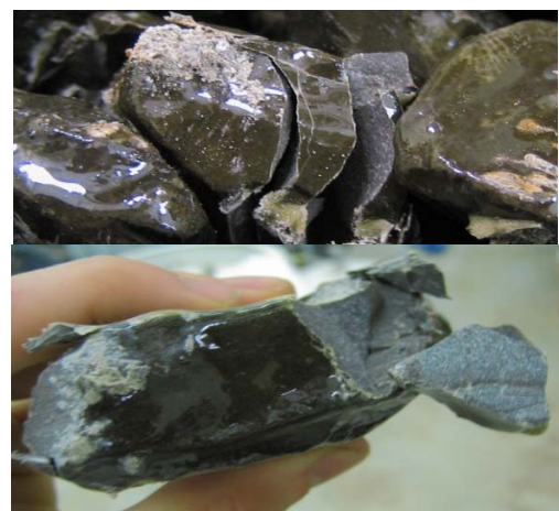
Figure 7 - Broken ballast still remained within the matrix via polyurethane coating.
