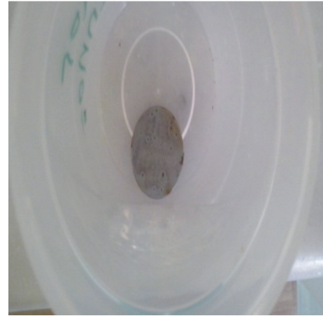
FIGURE 2: Withdrawn specimen. Note the significant corrosion of its surface.
