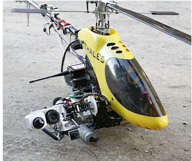
Figure 1. UAV platform with sensory payload consisting of 3 cameras; high-resolution, low-resolution and thermal
