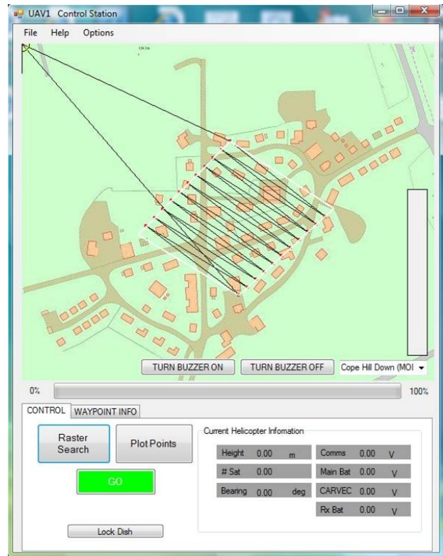
Figure 3. Mission control application, black lines indicate the flight path of the UAV over a village.
