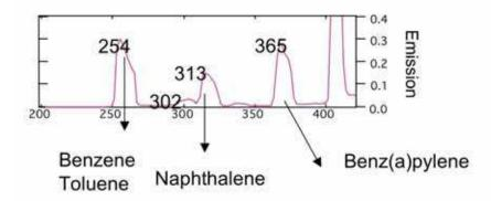
Fig. 15. The relation between the emission spectrum of mercury lamp and the  $\pi$ - $\pi$ \*absorption line of various aromatic VOCs.
