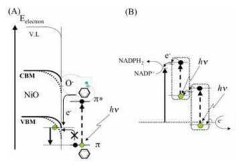
Fig. 9. The analogy between (A) VOC oxidation with the assist of photon energy and (B) light reaction (synthesis of reduction regent:  $NADPH_2$ ) in photosynthesis , which is named Z-scheme.
