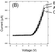
Fig. 7. The effect of acetone vapor introduction on the transport properties of a p-NiO/n-ZnO(Zn-face) heterojunction sensor element under dark. The current –time behavior at V=+4.5V forward bias is shown in figure (A). At the point (A), acetone vapor arrives at around the junction interface and after 600sec (point C) the acetone concentration reaches 4300ppm. The I-V curve B is that of point B in figure (A).
