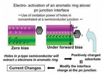
Fig. 2. The concept of "electro-" activation of combustible (reducing) gas molecules over a pn junction diode and its application to a chemical sensor.
