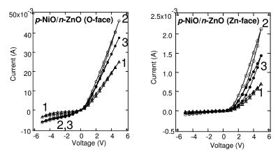
Fig. 10. The effect of toluene introduction on the I-V characteristics of a p-NiO/n-ZnO(Zn-face) and p-NiO/n-ZnO(O-face) heterojunction sensor elements. Curve 1: The I-V curve under dark, Curve 2: The I-V curve under UV light irradiation and Curve 3: The I-V curve in toluene 3325ppm atmosphere under UV light irradiation. Toluene sensing properties are added in both junctions under UV irradiation, though there are characteristic differences in the basic junction properties.
