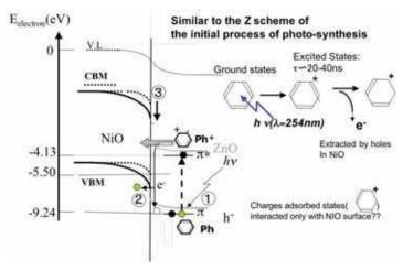
Fig. 3. Photo-driven oxidation process for aromatic VOCs over p-NiO surface under UV light incidence. Because of the large potential gap between VB edge of NiO and ground state of aromatic VOC (**Ph**), Ph is not oxidized under dark, however oxidation of exited state (=electron transfer from Ph\* to VB of NiO) is possible.
