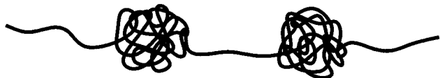
Figure 1. Schematic example of a necklacelike polymeric structure. Some regions of the chain adopt locally compact, globular conformations, while others exist in extended coillike states.
