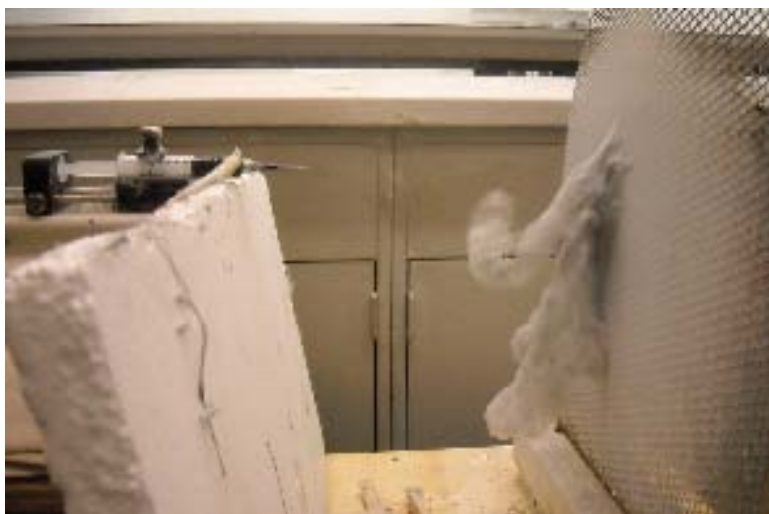
Figure 2: Photograph showing the electrospun nanofibers on the grounded collector.
