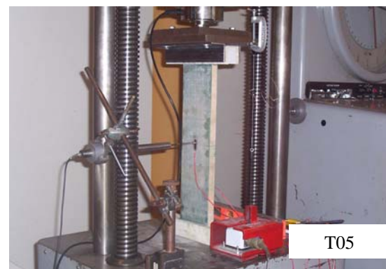
Figure 6. Columns test set-up
