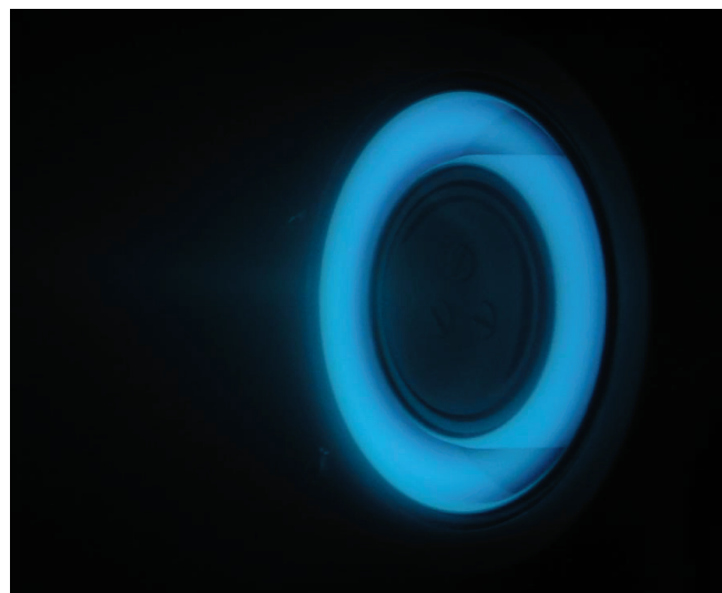
Figure 3. Operation of the MaSMi-60 at 250 V and 335 W showing evidence of successful magnetic shielding through a clear offset of the plasma from the inner and outer discharge channel walls.
