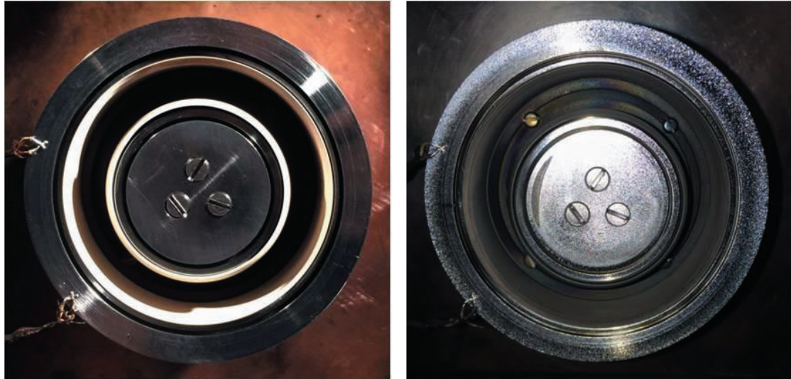
Figure 4. Comparison of the MaSMi-60's discharge channel and pole faces before and after ~ 20 hours of operation. Note the uniform layer of carbon deposited on the inner and outer channel walls, suggesting the presence of magnetic shielding, and the level of front inner and outer pole face erosion.
