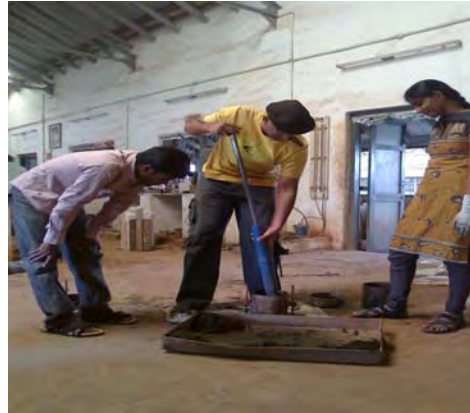
Plate 1. The Authors are conducting Modified Proctor Compaction Test
