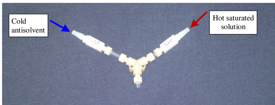
Fig. 2. Confined Y-shaped DIJ mixer configuration used in combined cooling-antisolvent crystallization experiments. This design allows for the convenient adjustment of jet velocity with implementation of Y-shaped mixers of different inner diameters with the same flangeless fitting connection.
