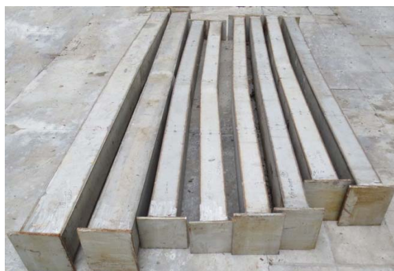
Fig. 9. Deformed shapes of all test specimens
