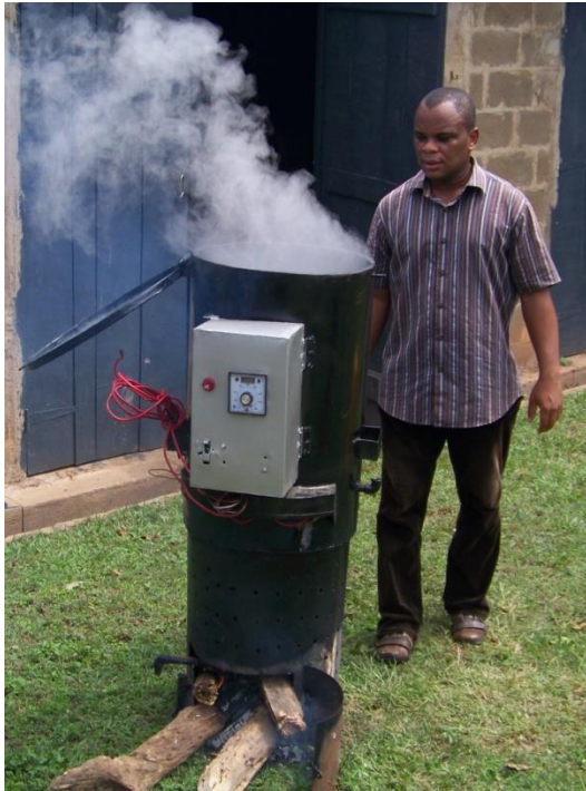
Plate 1 The dual-energy source steam boiler using firewood as a source of energy
