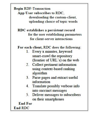
Figure 2: Top-Level Algorithm of System RDC
