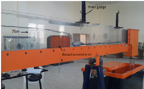
Fig. 2: Broad crested weir model
