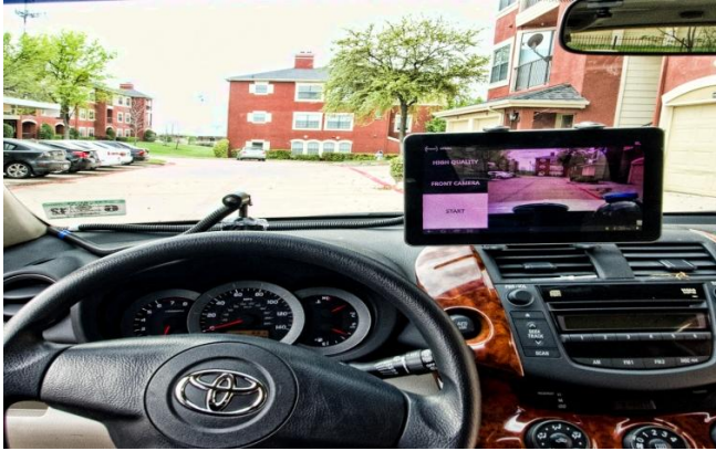
Fig. 3. A snapshot of inside the UTDrive data collection vehicle. The portable device is mounted on the wind-shield.
