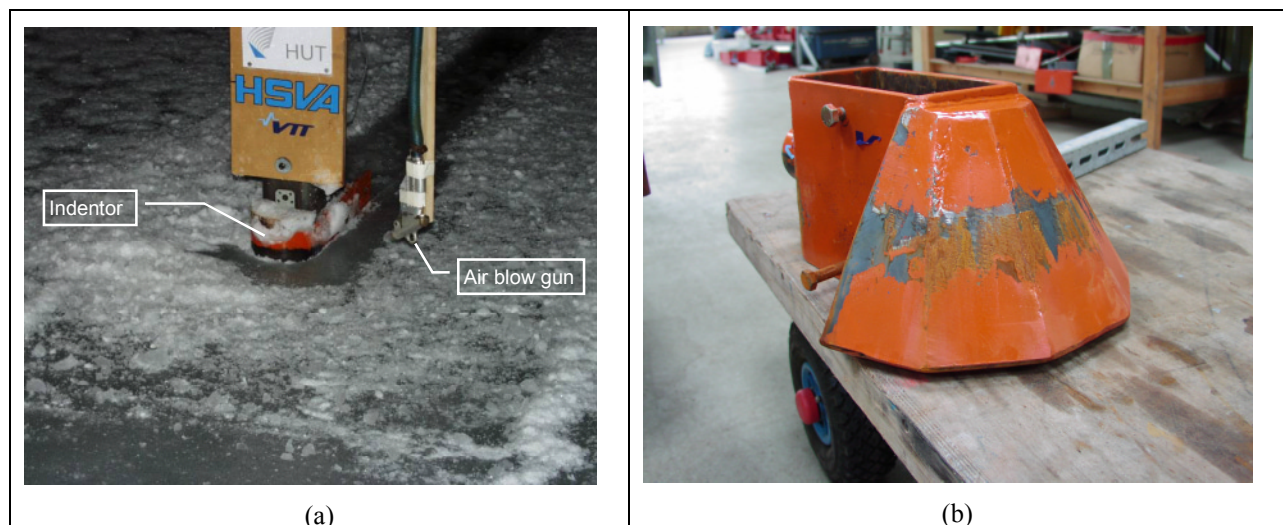
Figure 4. (a) Test set-up with a cylindrical indenter and an air blow system. (b) Conical indenter after the tests.
