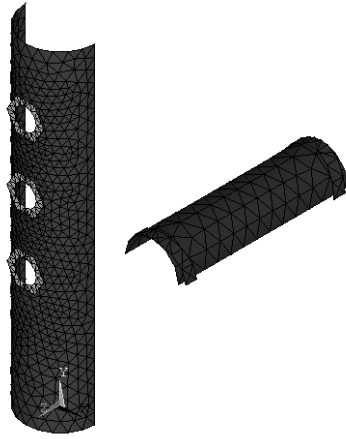
Fig. 9. Contact between bolts and tubes
