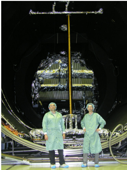
Fig. 9. TRP ULS project breadboard: boom with a 4.5m length.
