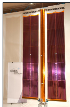
Fig.1. Solar array breadboard.
