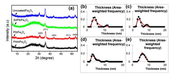
Fig. 2. (a) X-ray diffraction results of as synthesized Fe<sub>3</sub>O<sub>4</sub> nanoparticles. Area weighted thickness distribution of (b) Uncoated/Fe<sub>3</sub>O<sub>4</sub> (c) PAA/Fe<sub>3</sub>O<sub>4</sub> (d) PS/Fe<sub>3</sub>O<sub>4</sub> and (e) Si/PS/Fe<sub>3</sub>O<sub>4</sub> nanoparticles calculated by Mudmaster program and solid line (red) is the corresponding lognormal distribution fitting.
