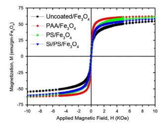
Fig. 8. DC magnetization curve scaled for per gram of Fe<sub>3</sub>O<sub>4</sub> nanoparticles.
