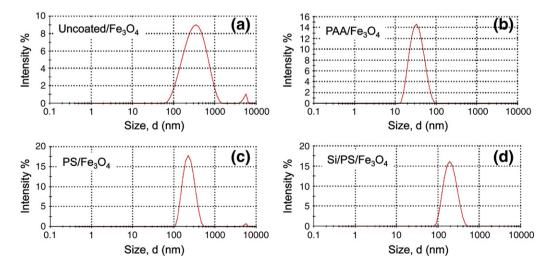
Fig. 4. Hydrodynamic size distribution of (a) Uncoated/Fe<sub>3</sub>O<sub>4</sub> (b) PAA/Fe<sub>3</sub>O<sub>4</sub> (c) PS/Fe<sub>3</sub>O<sub>4</sub> and (d) Si/PS/Fe<sub>3</sub>O<sub>4</sub> nanocomposites.
