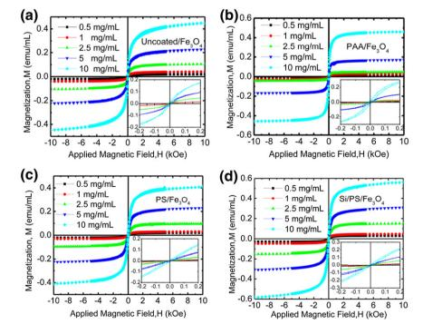
Fig. 6. DC magnetization curve from SQUID system for (a) Uncoated/Fe<sub>3</sub>O<sub>4</sub> (b) PAA/Fe<sub>3</sub>O<sub>4</sub> (c) PS/Fe<sub>3</sub>O<sub>4</sub> and (d) Si/PS/Fe<sub>3</sub>O<sub>4</sub> nanocomposite systems at different concentrations and inset shows the magnetization curve at a very low field.
