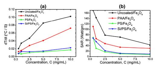
Fig. 10. (a) Initial heating rate of all samples at five different concentrations and (b) variation of SAR with respect to the nanoparticle concentrations.
