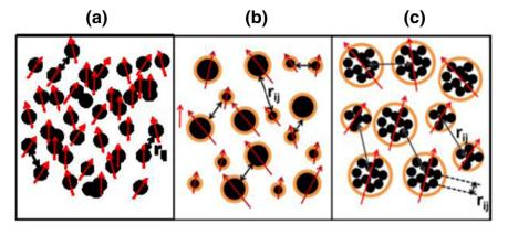
Fig. 12. Schematic diagram of the different nanoparticle system (a) representative of uncoated nanoparticles (b) nanoparticles coated with polymer (c) nanoparticles embedded in nanosphere matrix.
