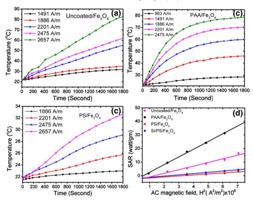
Fig. 13. Time dependent temperature curve at different AC magnetic field strength for (a) Uncoated/Fe<sub>3</sub>O<sub>4</sub> (b) PAA/Fe<sub>3</sub>O<sub>4</sub> and (c) PS/Fe<sub>3</sub>O<sub>4</sub> and (d) variation of SAR with square of AC magnetic field strength.
