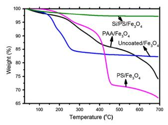
Fig. 5. Thermogravimetric analysis (TGA) results of different  $\mathrm{Fe}_3\mathrm{O}_4$  nanocomposite systems.
