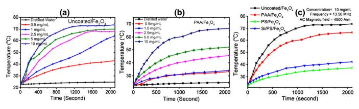
Fig. 9. Heating curve of (a) Uncoated/Fe<sub>3</sub>O<sub>4</sub> (b) PAA/Fe<sub>3</sub>O<sub>4</sub> at five different concentrations and (c) heating behavior of all four samples at a fixed concentration of 10 mg/mL.
