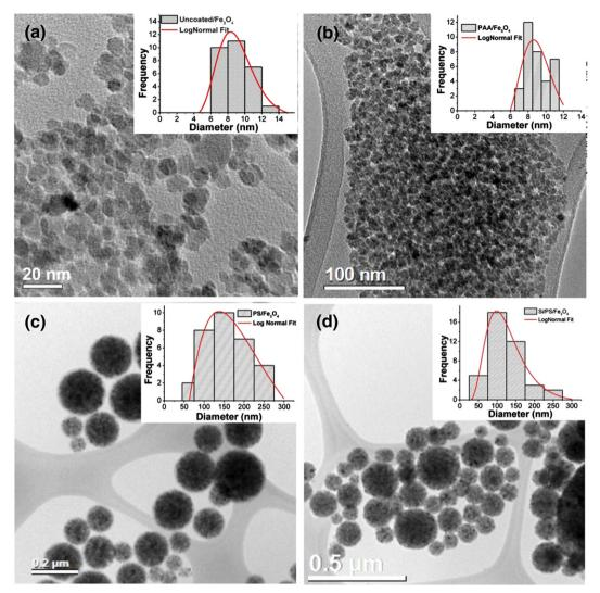
Fig. 3. Transmission electron microscopy image of (a) Uncoated/Fe<sub>3</sub>O<sub>4</sub> (b) PAA/Fe<sub>3</sub>O<sub>4</sub> (c) PS/Fe<sub>3</sub>O<sub>4</sub> and (d) Si/PS/Fe<sub>3</sub>O<sub>4</sub> nanocomposites and inset shows the corresponding histogram with log normal fitting.
