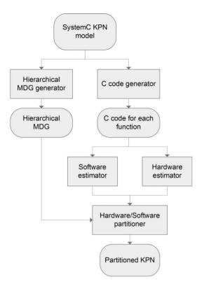
Figure 1. The KPN-based SoC design space exploration flow.
