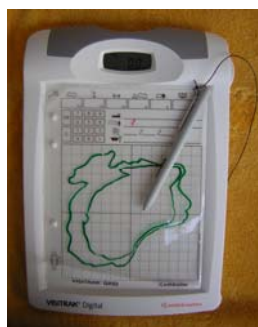
Figure 2. The instrument Visitrak Digital used to measure eschar surface area
