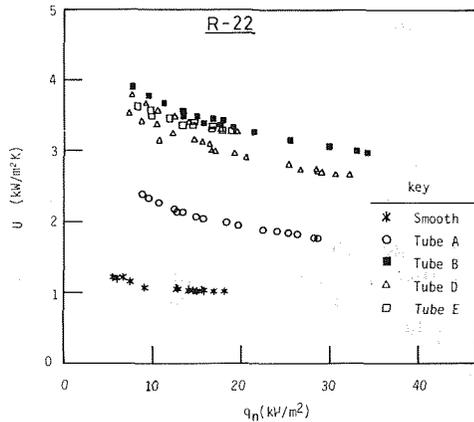
Fig. 9 Overall heat transfer coefficient versus heat duty
