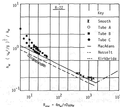
Fig. 8 Variation of nondimensional condensing heat transfer coefficient with film Reynolds number
