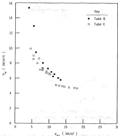
Fig. 6 Cross-check test for condensing heat transfer coefficient
