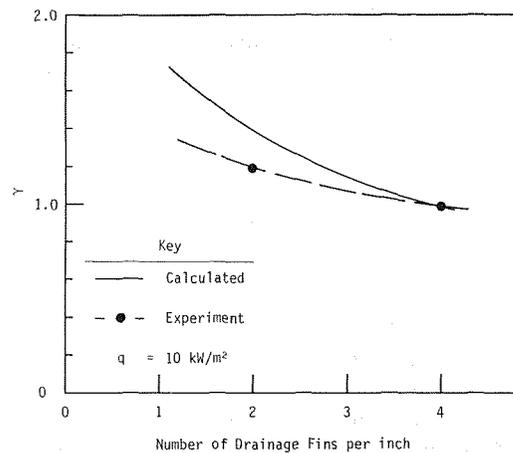
Fig. 7 Effect of the pitch of spiral on condensing heat transfer performance
