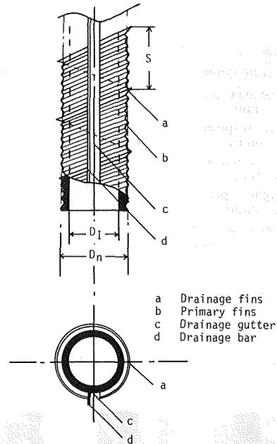
Fig. 3 Schematic cross-sectional view of test tube
