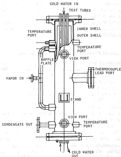
Fig. 2 Schematic diagram of condenser
