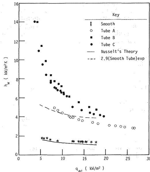
**Fig. 5 Condensing heat transfer coefficient for smooth tube, Tube A, Tube B, and Tube C**
