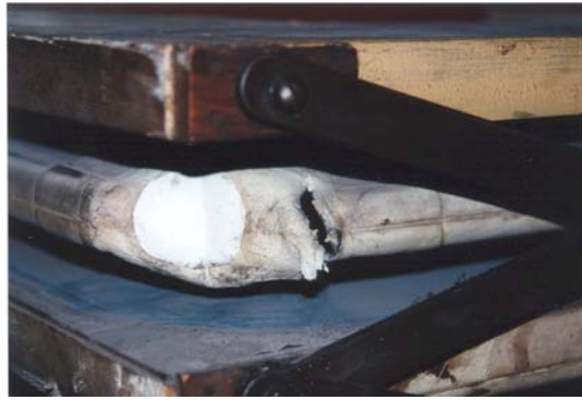
Figure 2. Damage to bellows
