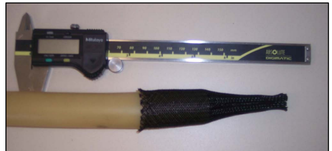
Figure 3. Section of \frac{5}{8} in. Braid set over 25.4 mm (1 in.) tube. PAMs with smaller diameter braids had smaller braid angles.
