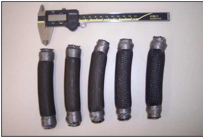
Figure 4. From left to right, PAMs with braid angles of 40.9°, 38.10°, 58.57°, 60.51°, and 67.36°.
