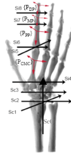
Fig. 6 Frames defining links along the index finger
