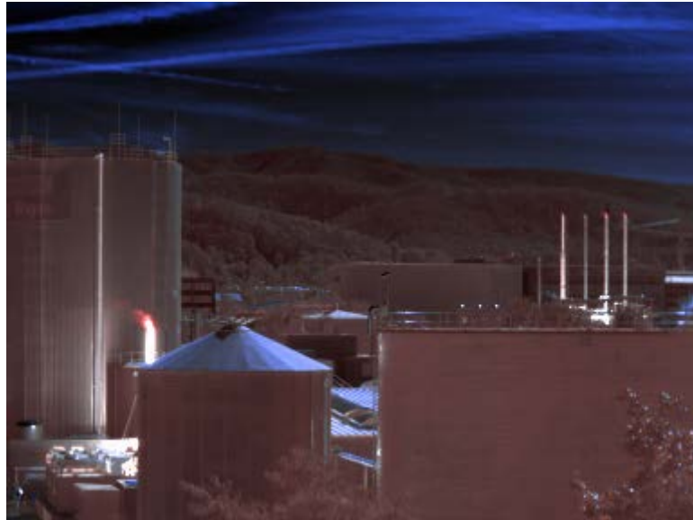
Fig. 7. Bispectral IR image of an industrial area by a superposition of the two individual channels in a blue and a red color scale, respectively. The signatures of CO 2 emissions of smokestacks appear in red.
