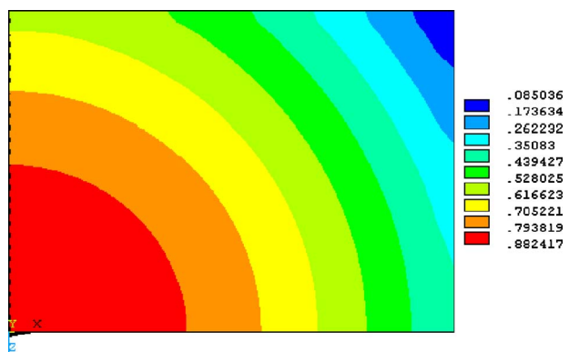
Fig. 16 Strain \varepsilon_y in the TIM at the reflow temperature (loadstep 4)
