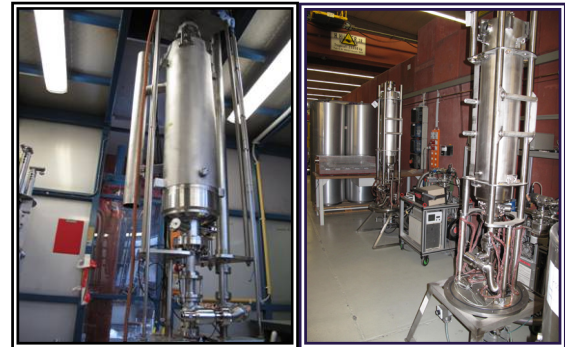
Figure 1: Left side: Cavity equipped with helium tank and all accessories installed to the vertical test insert. Right side: Cavity dressed with helium tank installed to 120°C baking apparatus before vertical RF measurement.
