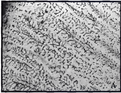
Fig. 8 — A — Microstructure of clad metal, unsteered, 1050 A, 100X; B — microstructure of clad metal, steered, 1050 A, 100X.
