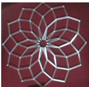
Figure 13. A multi-segmented assembly of a radially foldable planar linkage.
