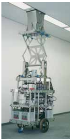
Fig.1 Air Conditioning Equipment Inspection Robot
