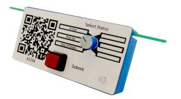
**Figure 1:** An RF-powered Arfid prototype controller supporting pushbutton and rotary-dial input modalities. Users scan the QR code to configure, via a web interface, the function that the tactile input controls for each individual device.
