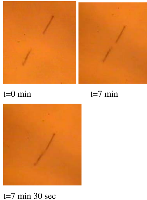
Figure 5. Attraction between two floating rods in the presence of the electric field. The device shown in figure 1 is subjected to a voltage of 5000 V. The other parameters are the same as in figure 3. As the rods come closer, they align along the line joining their centers. They maintain this orientation until touching.
