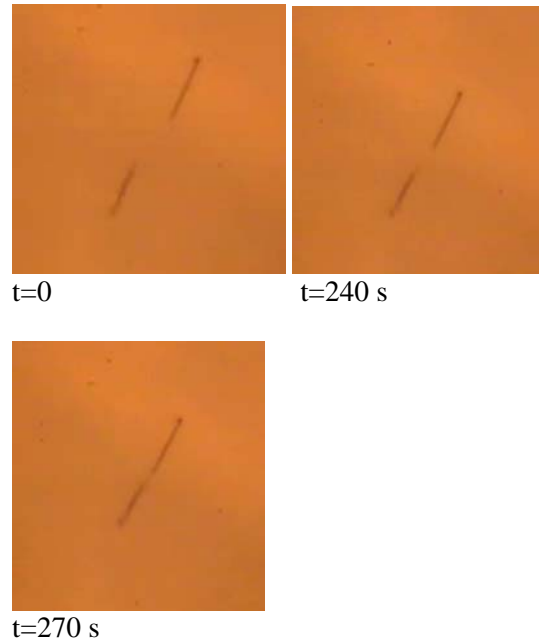
Figure 3. Attraction between two floating rods. The parameters are the same as in figure 2. The electric field is still turned off. Initially, the rods are approximately parallel to the line joining their centers. As they come closer, they align so that they are approximately parallel to the line joining their centers. In their final equilibrium position, the rods maintain this orientation and touch each other.
