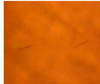
Figure 9. Attraction between two floating rods in presence of an electric field. The voltage applied is 5000 V. The remaining parameters are the same as in figure 2. Initially, the rods are approximately perpendicular to each other. However, they rotate to become approximately parallel to the line joining their centers. The rods' behavior being the same as in figure 3 after t=360 min, the dynamics after that time is not reproduced here.
