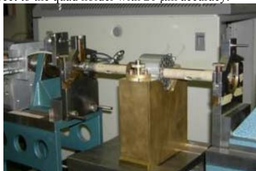
Figure 1: CERN magnetic measurement bench with \text{SmCo}_5 quadrupole prototype.
