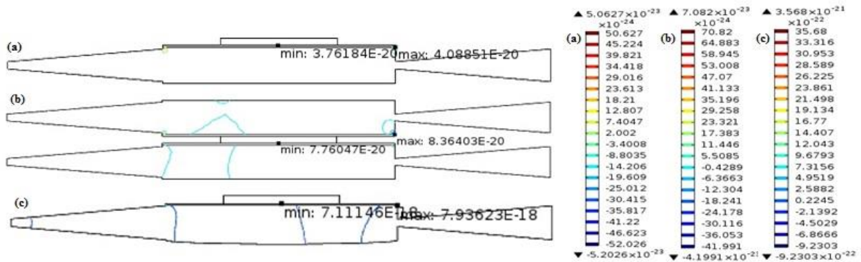
Figure 4. Pressure distribution in the different parts of the micro-pumps
