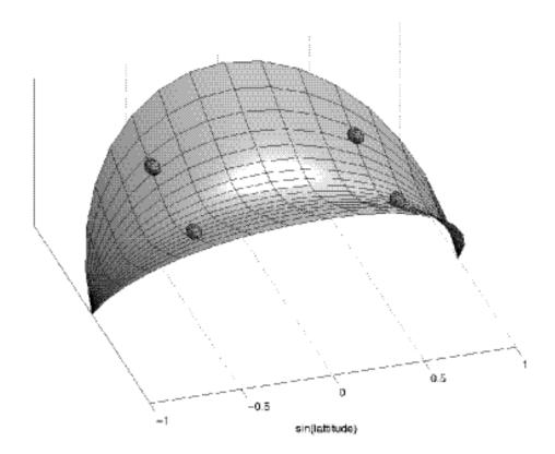
Fig. 1. The geometry of the meridional, parabolic, channel on the spherical earth. The spherical earth itself is missing from the figure and only the channel is portrayed. The longitude scale is arbitrary (bottom shoaling depends on ) and the vertical axis is the height from the earth's center i.e. the ratio of channel's depth to earth's radius is greatly exaggerated.
