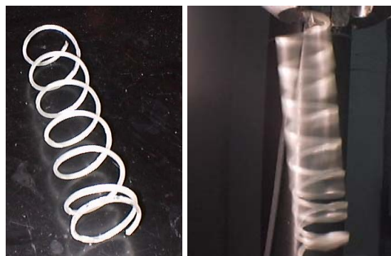
Figure 1. A composite helical spring made with glass strands (left), and the same spring at its 28.25 Hz resonant frequency (right).
