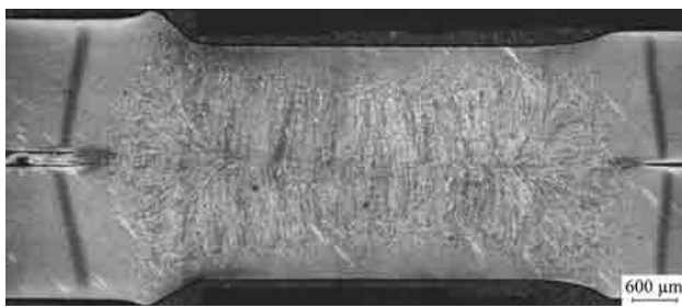
Fig. 3 - RSW welding spot between DP steel sheets. Axial metallographic section. Light microscope.
