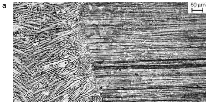
Fig. 13 - Simulated LW welding line in a TWIP steel sheet. Transversal metallographic section (a) and magnification (b). Light Microscope.
